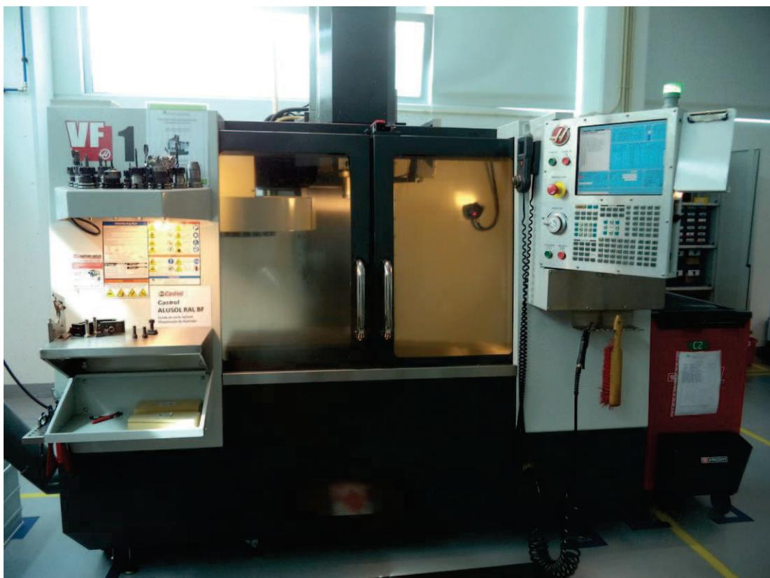
Figura 5 – Fresadora CNC HAAS VF 1
